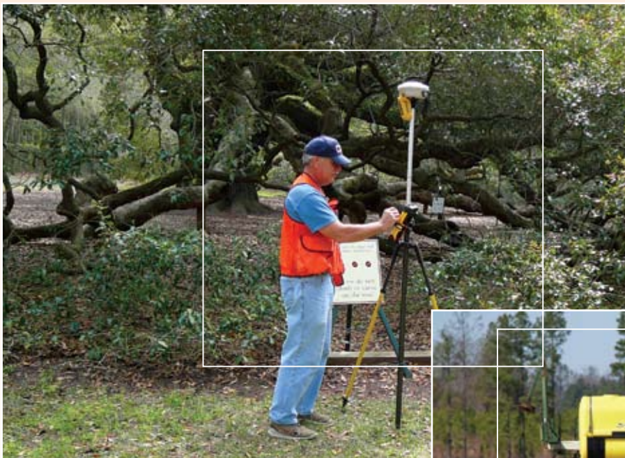
▲ Dr. Lew Lapine, PLS uses a GNSS receiver within the SCVRS network to obtain orthometric heights as quality control for a lidar survey in Charleston County, South Carolina. He stands in front of South Carolina's largest live oak tree, known as Angel Oak, over 1,500 years old and supposedly the oldest living thing east of the Rockies.
